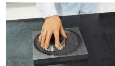
Lapping - precision finishing of spacer faces on a lapping machine
