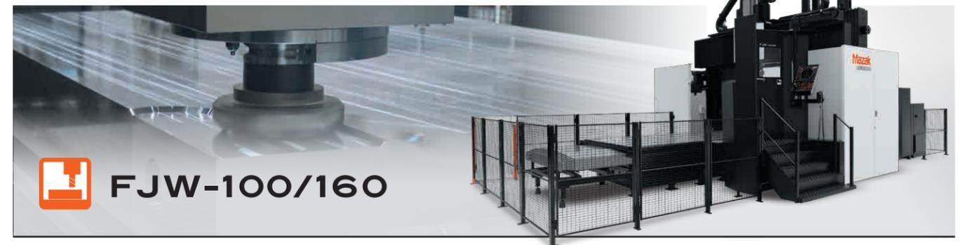
FJW-100/160 is a double-column vertical machining center suitable for large-sized workpieces that require 5 face machining such as parts used in semiconductor production equipment and other industrial machines. Equipped with a 6000 rpm high torque 828 N·m (611 ft·lbs) spindle, the machining center can handle the heavy-duty cutting of steel, cast iron, etc. In addition to the high rigidity double-column structure, powerful machining can be performed by utilizing slide ways on Y-axis and
