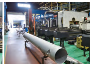
Pipes up to a maximum of 406.4 mm in diameter can be processed
