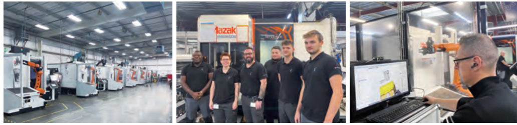
Highly automated cell in Alabama consisting of Mazak machines coupled with robotic arms
