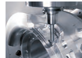
5-axis machining center is machining the upper and inclined surface at once
