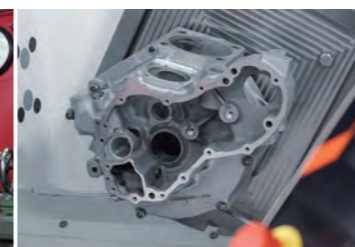
Internal combustion engine machined with VARIAXIS j-500/5X
